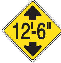
Vehicles or loads higher than the clearance shown can't go through the underpass.
