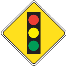
Traffic signal ahead. Be prepared to stop.
